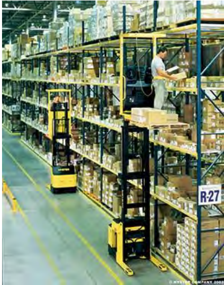
Fig 2.4.22: Operating at more than 1 meter from the ground
