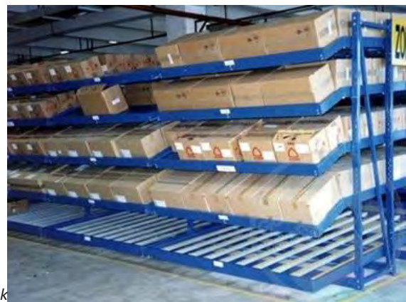
Fig 1.3.15: Gravity Flow Rack
