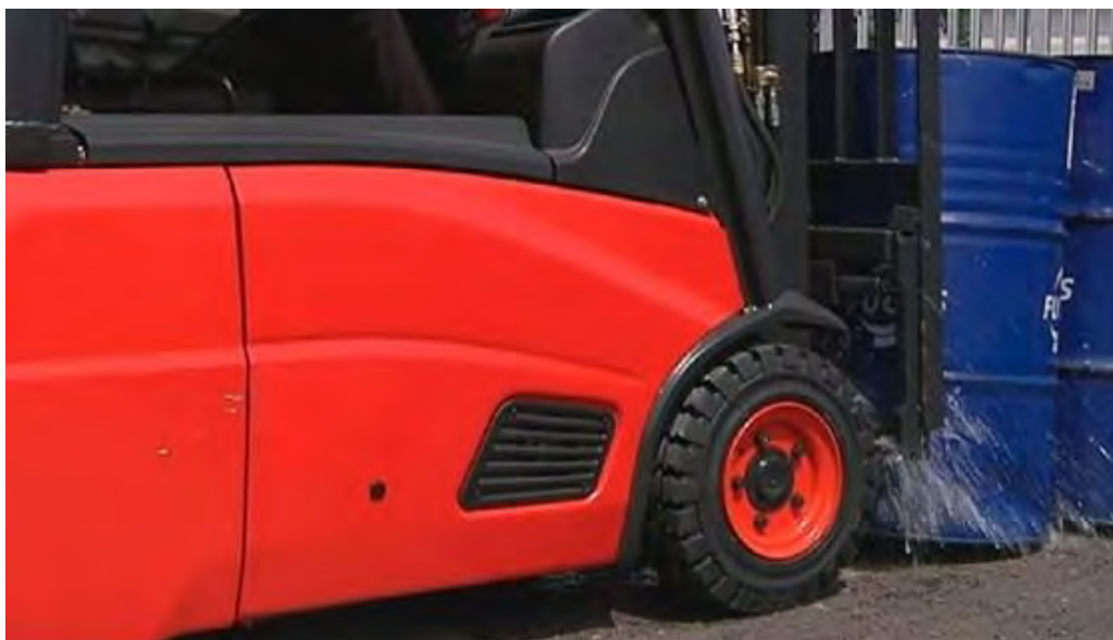
Fig 5.2.72: Forklift equipment causing damage
