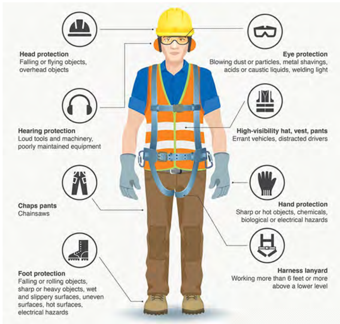
Fig. 2.3.3. Identification of Safety Gears
