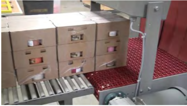
Fig. 2.3.5. Shrinking Machine and Shrink Wrapped Cargo
